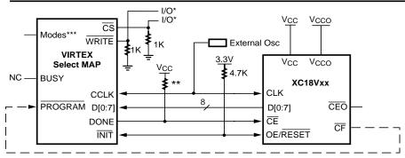
$<sup>^*\</sup>overline{\text{CS}}$  and  $\overline{\text{WRITE}}$  must be pulled down to be used as I/O. One option is shown.  $^**\text{Virtex}$ , Virtex-E is 300 ohms, all others are 4.7K.
