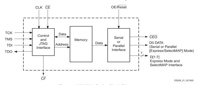
Figure 1: XQ18V04 Series Block Diagram
