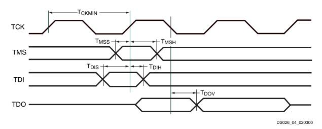
Figure 4: Test Access Port Timing
